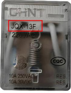
The image shows a CHNT JQX-13F relay component. The model number 'JQX-13F' is highlighted with a red box. Other markings include '220VAC', '10A 250VAC', '10A 30VDC', 'RES. RES.', and the CQC logo. |
